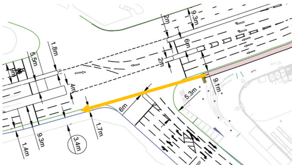
Extract of drawing PB9144-RHD-GE-SW-DR-R-0096 S3 P16 showing cycle movement across Syon Lane/ A4 junction
