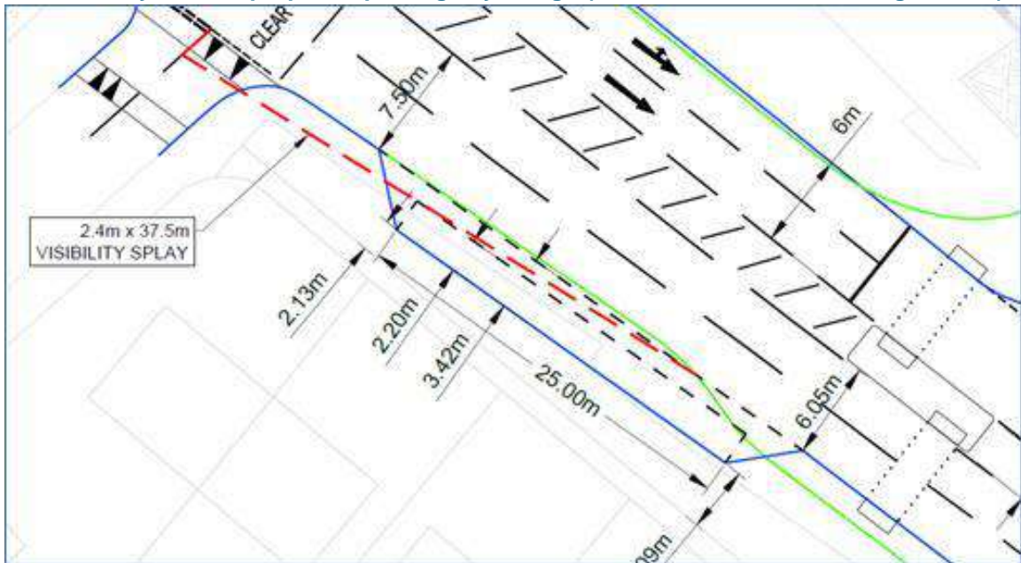
Insert 9.4: Syon Lane proposed parking bay design (amended as a result of Stage 1 RSA)
