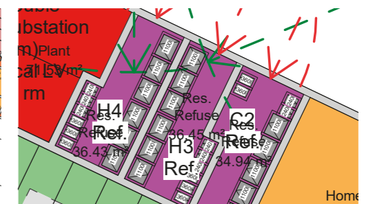
All refuse stores sized for capacity of waste streams and unit sizes as HBC policy, including provision for allocated areas of bulky waste.
